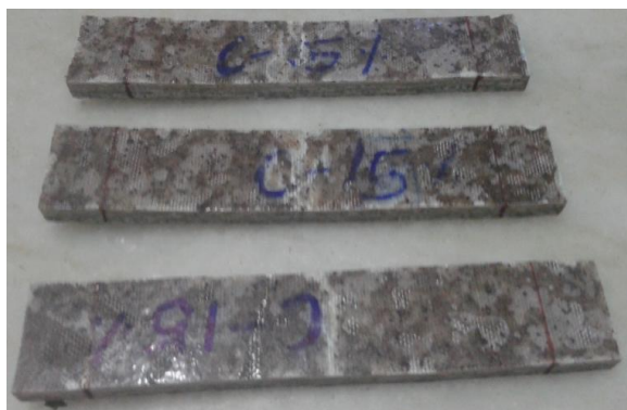
Fig. 6 Flexural strength tested specimens
