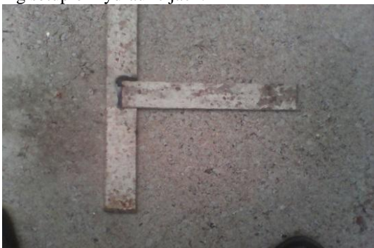
Fig 3.1 Test Specimen of Unsymmetrical Weldment
