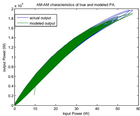
Fig.1: Comparison of AM/AM characteristics of actual and modeled PA
