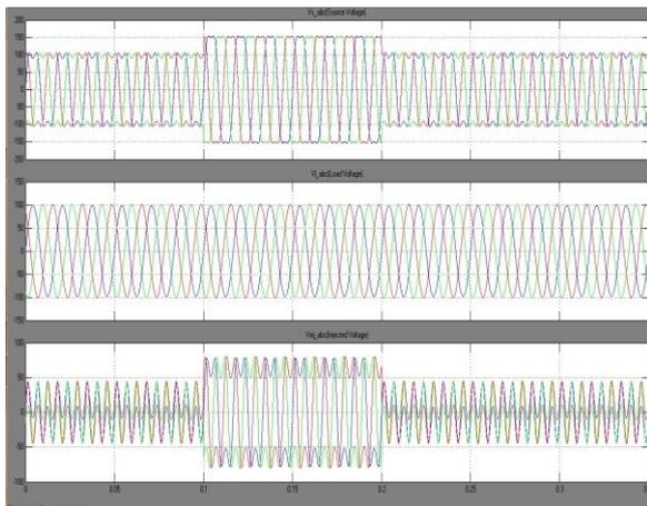
Fig.11.input Voltage, Load Voltage and Injected Voltage with Swell condition
