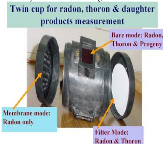
**Figure 1.**Radon-Thoron mixed field dosimeter system.
