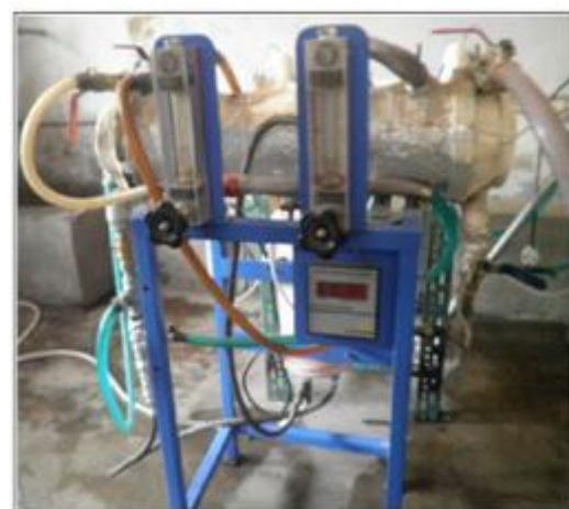
Fig.2: Straight tube heat exchanger Experimental setup
