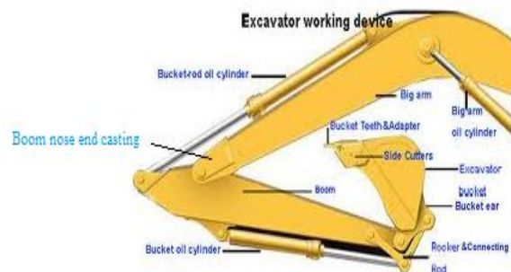
Figure I.1: Excavator with different parts
