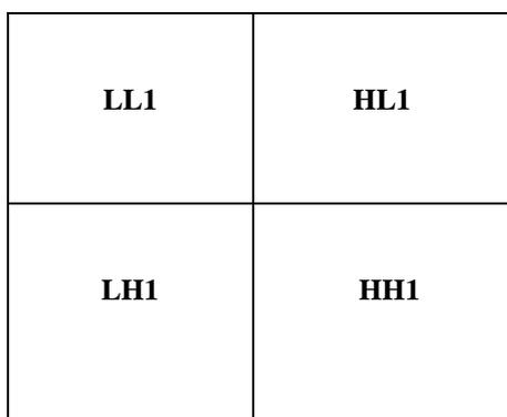
Fig. 6: DWT Decomposition with Level-1.
