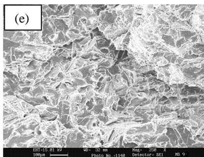
Fig 7a,b,c & d: Fractographs of cryogenically solidified nano metal matrix composites 3 Wt. % to 12 Wt. % of reinforcement using 15 mm copper end chill thickness at 500X magnification and scale 100  $\mu\text{m}$ . Fig 7e factograph of cryogenically solidified metal matrix material (LM13).
