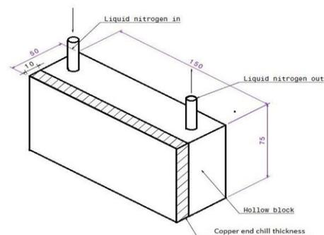
Fig. 2: Copper end chill in a steel hollow block (Brazed) for passing liquid nitrogen
