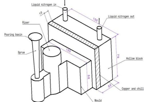
Fig. 1: Sand mould with Copper end chill with arrangements for passing liquid nitrogen
