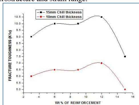
Fig 6: Graph shows the Wt% of reinforcement v/s Fracture toughness (K1c).
