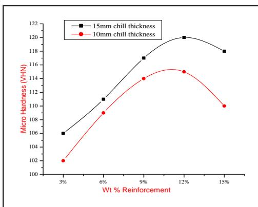
Fig. 4: Graph showing Wt % of reinforcement v/s Vickers Micro Hardness Test
