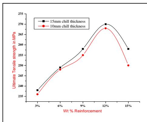
Fig. 5: Graph showing Wt % of reinforcement v/s UTS
