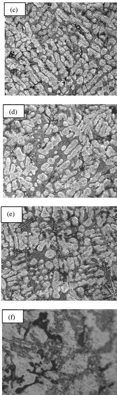
Fig. 3a: LM13 Al alloy ingot, Fig. 3b: 3 Wt% of Nano ZrO<sub>2</sub>, Fig. 3c: 6 Wt% of Nano ZrO<sub>2</sub>, Fig. 3d: 9 Wt% of Nano ZrO<sub>2</sub>, Fig. 3e: 12 Wt% of Nano ZrO<sub>2</sub> & Fig. 3f: 15 Wt% of Nano ZrO<sub>2</sub>. Micro Structure taken at 100X magnification.
