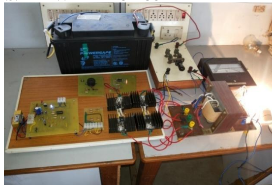
Fig.6. Assembled Prototype of inverter circuit
