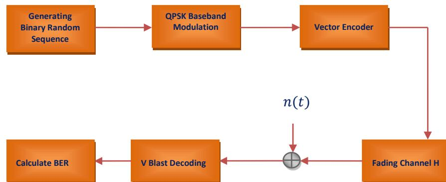
Fig 4: Simulation Process of V-BLAST
