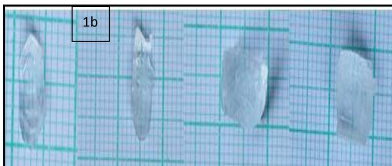
**Figure 1:** (a) Solubility curve; (b) (from left to right) Photograph of BTCBC; LA<sub>0.3</sub>BTCBC<sub>0.7</sub>; LA<sub>0.5</sub>BTCBC<sub>0.5</sub>; and LA<sub>0.7</sub>BTCBC<sub>0.3</sub> single crystals.
