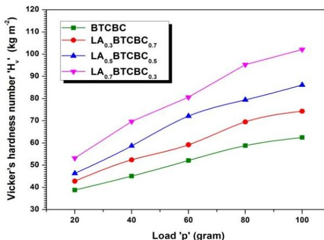
**Figure 4:** Variation of  $H_v$  with load for pure and L-alanine mixed BTCBC single crystals
