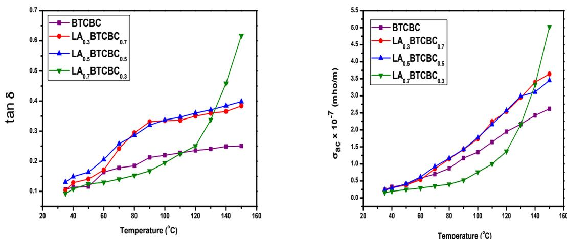
**Figure 7:** Variation of loss factor and AC conductivity with temperature for pure and L-alanine mixed BTCBC single crystals
