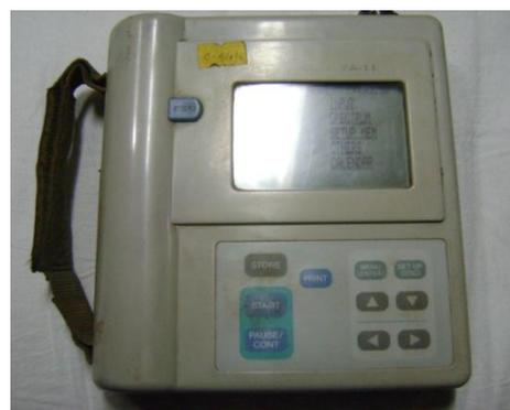
**Figure 5 - Vibration Analyzer**
