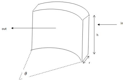
Fig 1 Schematic of control volume showing mass entry and exit through a differential radius
