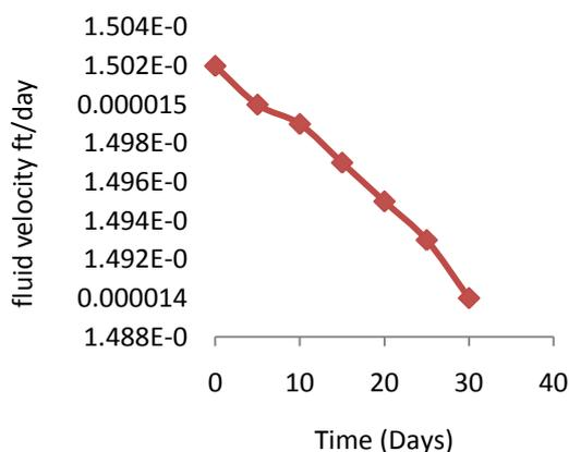
Fig 5 plot of oil velocity against time
