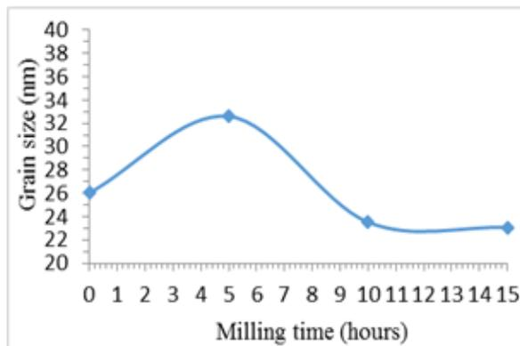
Fig.5 Variation of grain size of Al-Fe-Cr-20 wt. %  $Al_2O_3$  composites with different milling time.
