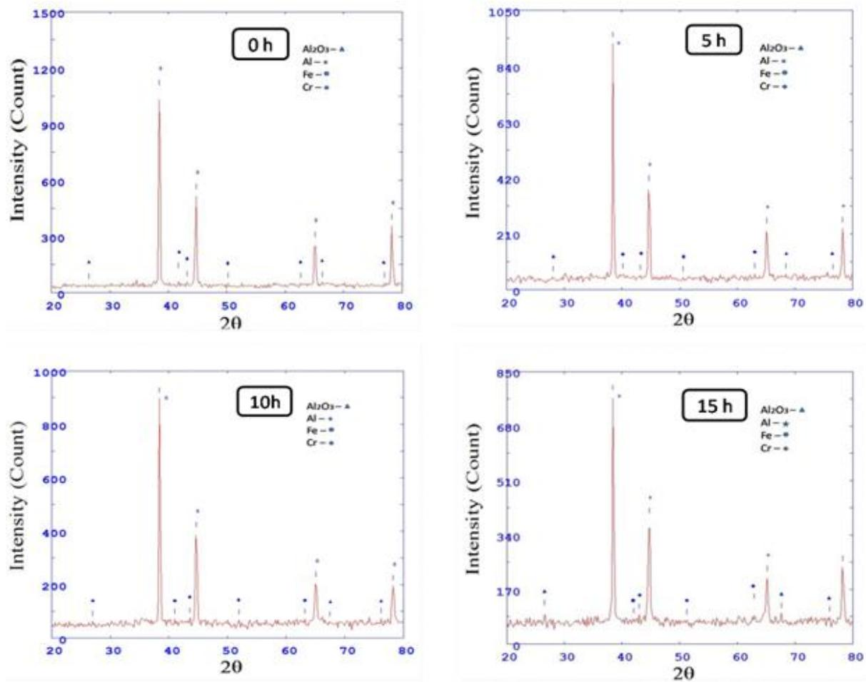
Fig. 4 XRD patterns of Al-Fe-Cr-20 wt. %  $Al_2O_3$  composite powder after (a) 0 h, (b) 5 h, (c) 10 h and (d) 15 h of ball milling.
