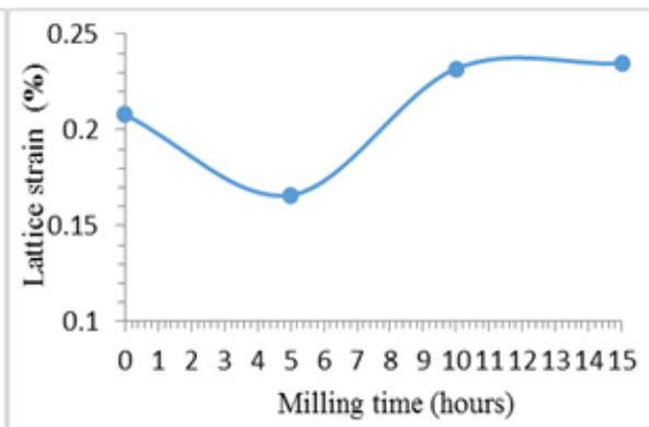
Fig.6 Effect of milling time on lattice strain of Al-Fe-Cr-20 wt. %  $Al_2O_3$  composites.
