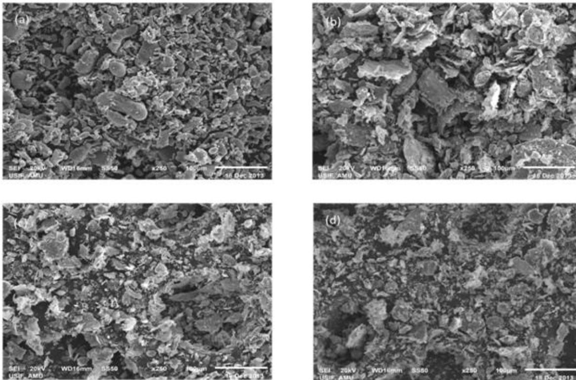
Fig. 2 SEM images of Al-Fe-Cr-20 wt. % Al<sub>2</sub>O<sub>3</sub> composite powder after (a) 0 h, (b) 5 h, (c) 10 h and (d) 15 h of ball milling.
