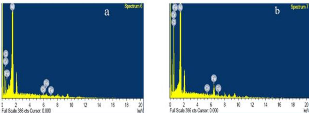
Fig. 3 EDX patterns of Al-Fe-Cr-20 wt. % Al<sub>2</sub>O<sub>3</sub> composite powders ball milled for (a) 0 h and (b) 15 h.
