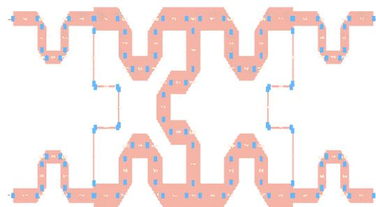
Fig.7. Fractal-shaped 3-section branch line coupler
