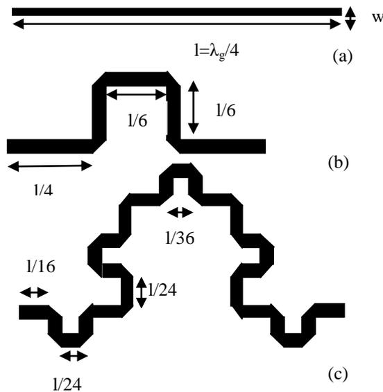
Fig 6. Koch-shaped micro-strip-line with iteration factor of 1/4
