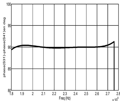
Fig 3. Phase difference between the two output ports
