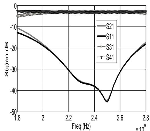
Fig.8. Simulated results of the designed 3-section fractal branch line coupler
