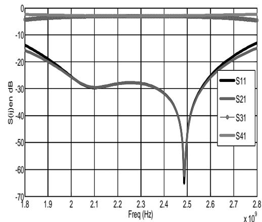
Fig.2. Simulated results of the designed 3-section branch line coupler
