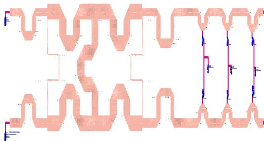
Fig.10. layout 2bits fractal phase shifter
