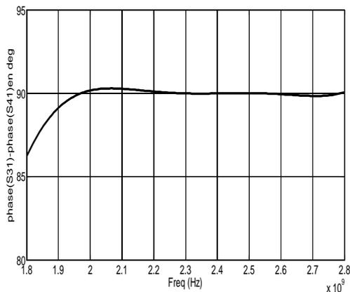
Fig 9. Phase difference between the two output ports
