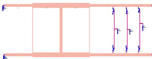
Fig.4. Layout 2bits phase shifter with 3section coupler
