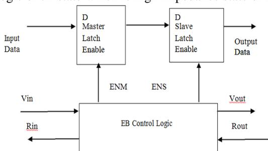
Figure 3: Elastic Buffer using D flip-flop [1]
