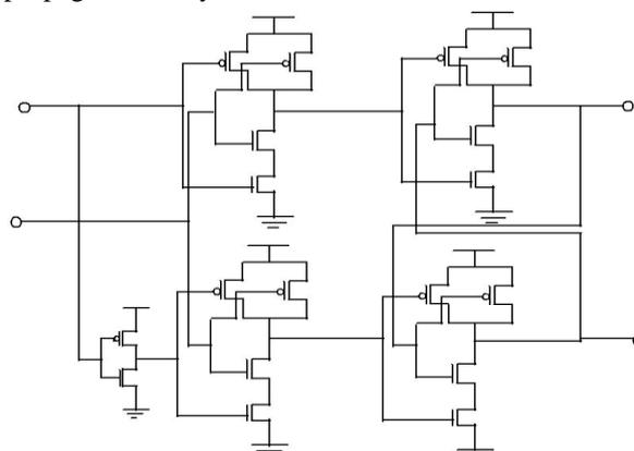
Figure 1: D Flip-Flop [2]
