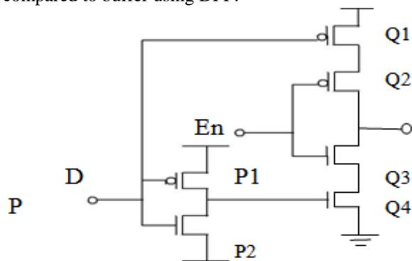
Figure 2: Tri-state Buffer [2]
