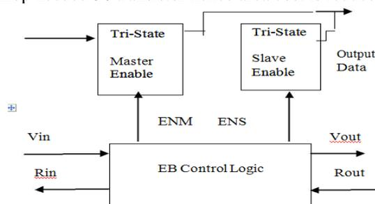
Figure 4 : Master slave tri-state buffer with control logic
