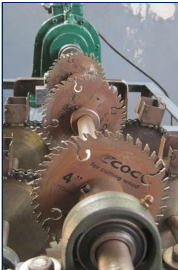
Fig.13 Cutters held on shaft by the sleeves
