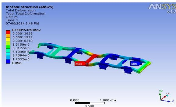
Figure 18: Total Deformation for steel
