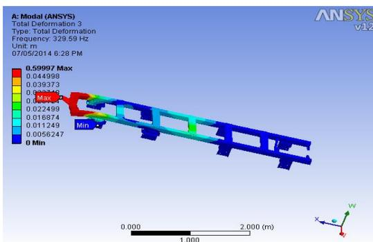
Figure 6: Deformation (Third Mode)
