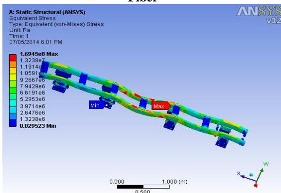
Figure 19: Equivalent (Von Mises) Stress for Carbon Fiber material
