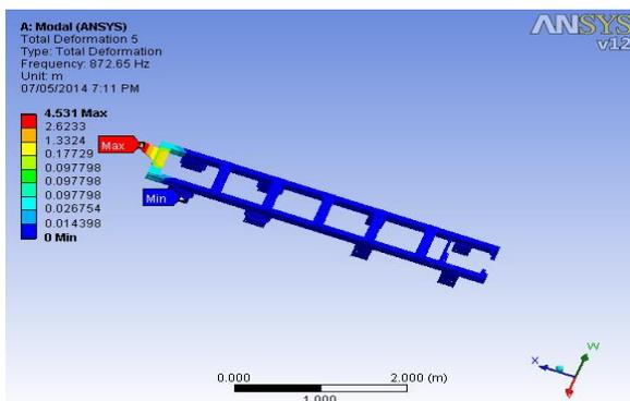
Figure 14: Deformation (Fifth Mode)
