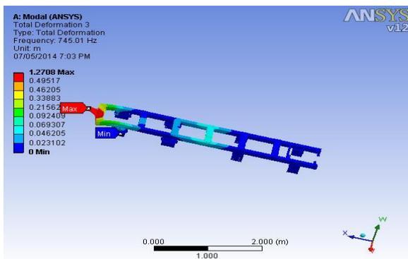
Figure 12: Deformation (Third Mode)
