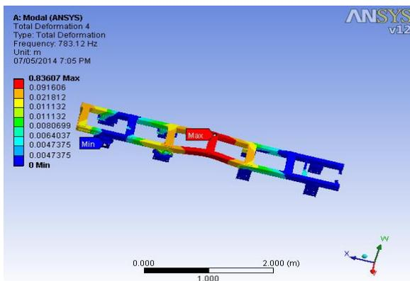
Figure 13: Deformation (Fourth Mode)
