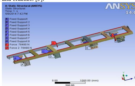
Figure 3: After applying the boundary conditions
