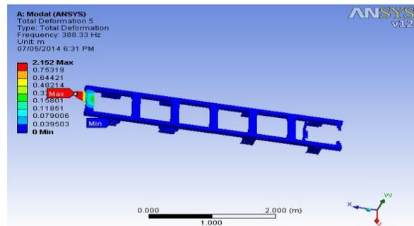
Figure 8: Deformation (Fifth mode)
