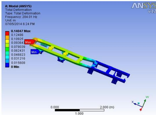
Figure 4: Deformation (First mode)
