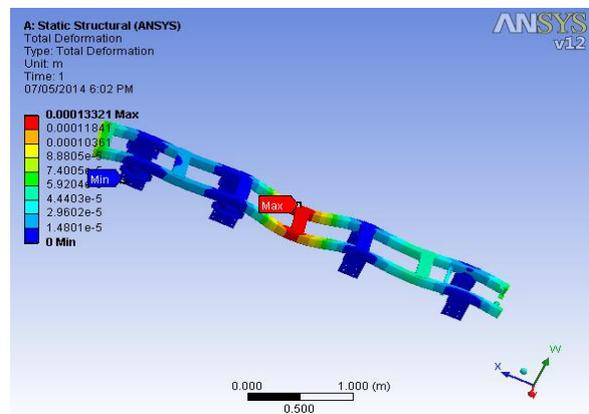
Figure21: Total deformation for Carbon Fiber material
