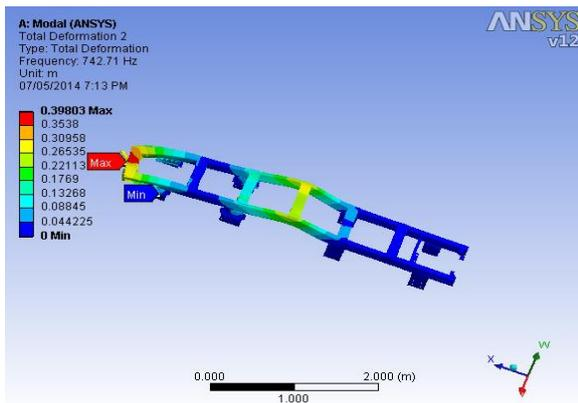
Figure 11: Deformation (Second Mode)
