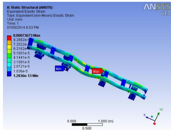
Figure 20: Equivalent (Von Mises) Strain for Carbon Fiber material
