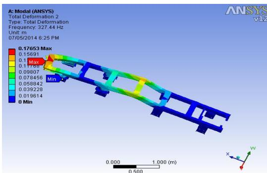
Figure 5: Deformation (Second Mode)
