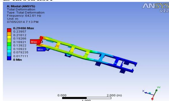
Figure 10: Deformation (First Mode)
