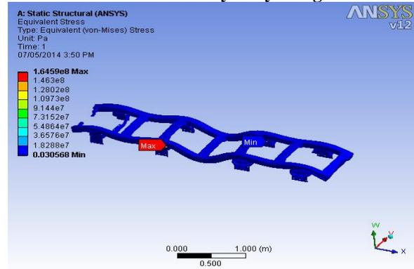
Figure 16: Equivalent (Von Mises) Stress for steel
