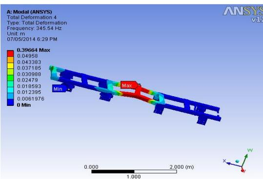
Figure 7: Deformation (Fourth Mode)
