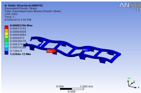
Figure17: Equivalent (Von Mises) Strain for steel
