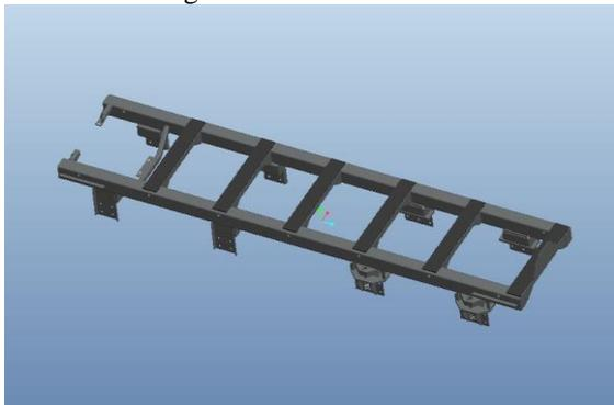
Figure 1: Solid model of fire truck chassis
