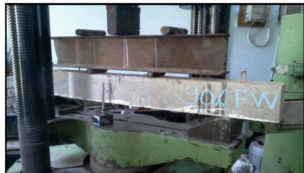
Fig. 2 beam test setup
