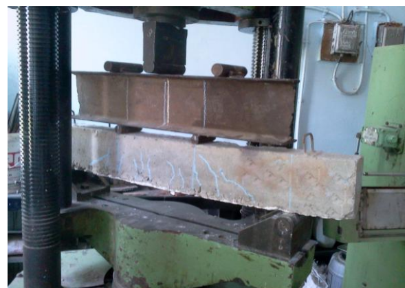
Fig. 8 cracking pattern for the control beam
