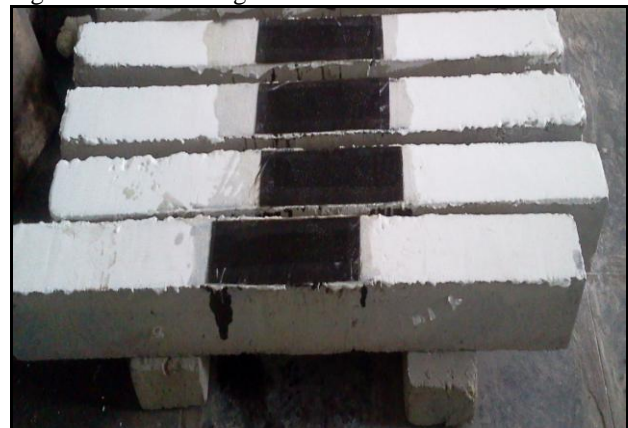
Fig. 3 application of sheets
