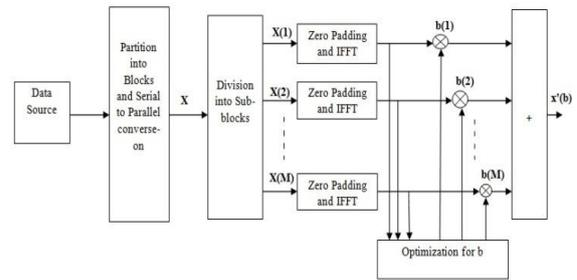
Fig.4 Block diagram of PTS technique
