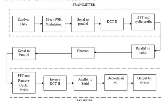
Fig.1 OFDM Model using DCT-II
