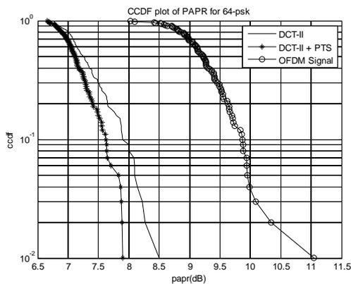
Fig.6 CCDF plot of PAPR for 64-PSK
