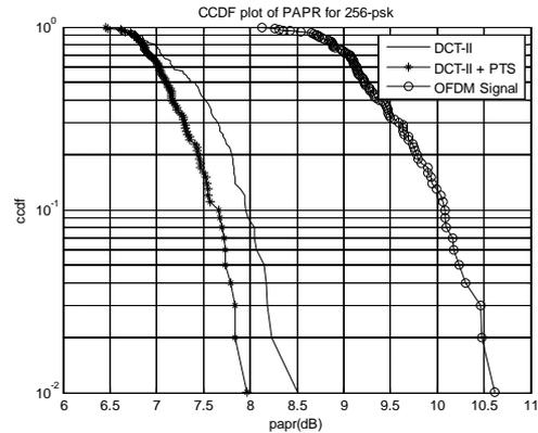
Fig.8 CCDF plot of PAPR for 256-PSK
