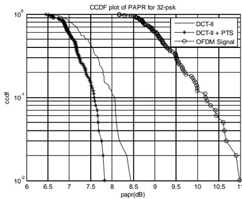
Fig.5 CCDF plot of PAPR for 32-PSK
