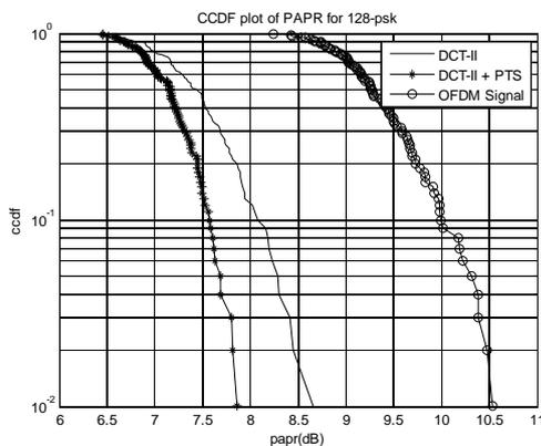
Fig.7 CCDF plot of PAPR for 128-PSK
