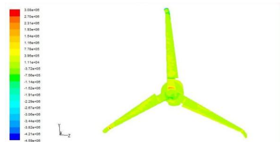
Figure 3.8 Static Pressure for Wind speed 4.0 m/s
