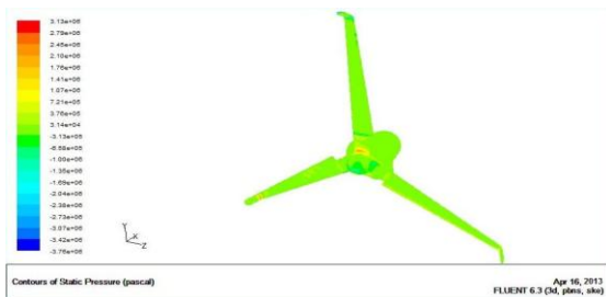
Figure 3.2 Static Pressure for Wind speed 2.0 m/s
