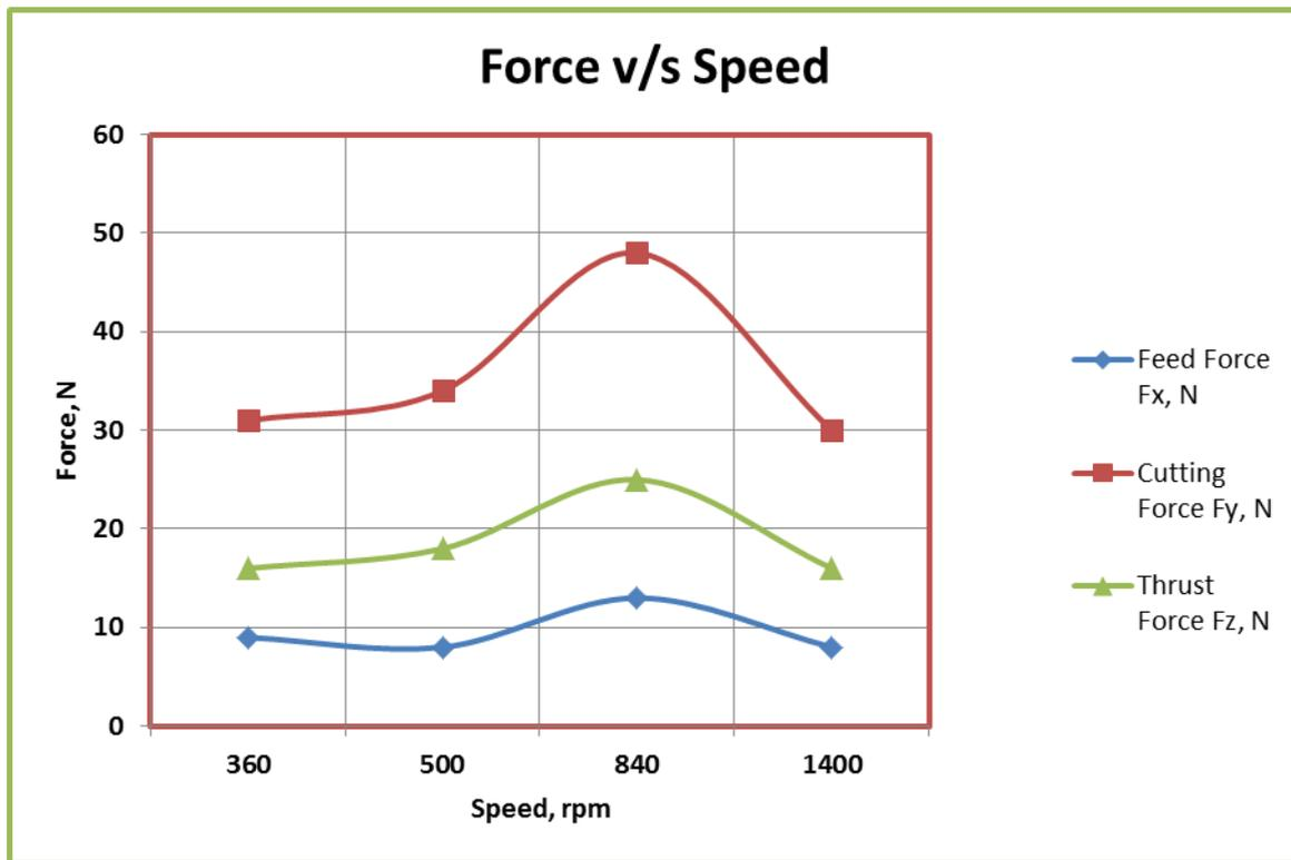
Figure 5. Force v/s Speed curve for constant depth of cut
