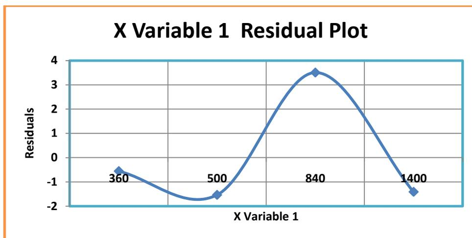
Figure6. Residual Plot for Feed Force,  $F_x$  HSS Tool
