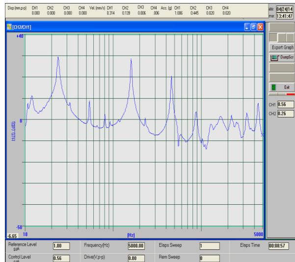
Fig. 6 Variation of transfer function with Frequency for steel beam
