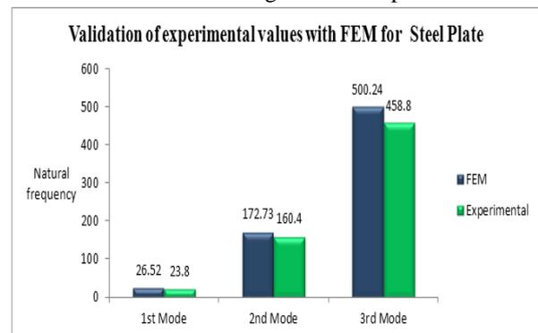
Fig. 7 Comparisons of experimental results with FEM for Steel Plate
