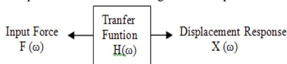
Fig. 1 Frequency Response Function (FRF)
