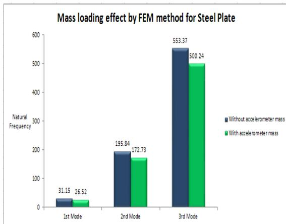
Fig. 4 Accelerometer mass loading effect on Steel Beam
