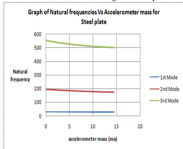
Fig.3 Variation of natural frequencies with accelerometer mass for Steel Plate
