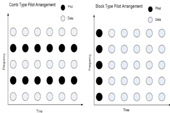
Fig.2 Block Type & Comb Type Pilot Arrangement
