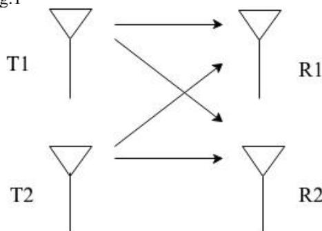
Fig. 1 MIMO-OFDM System with two transmitting antenna and two receiving antenna
