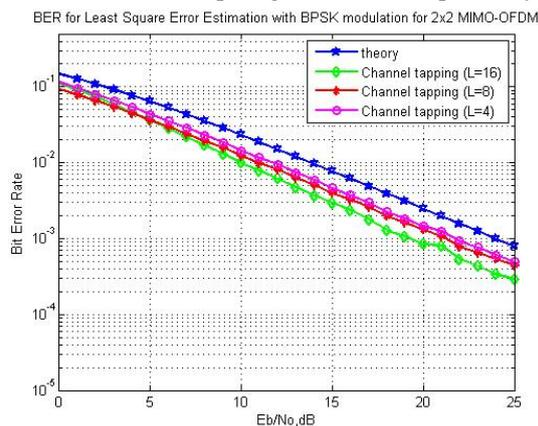
Fig. 3 BER performance comparisons for different channel tapping lengths by using Least Square (LS) estimation technique for  $2 \times 2$  MIMO-OFDM
