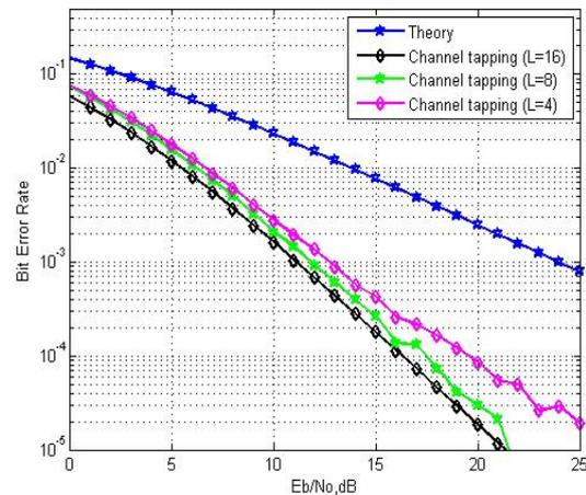
Fig.4 BER performance comparisons for different channel tapping lengths by using Minimum Mean Square (MMSE) estimation technique for  $2 \times 2$  MIMO-OFDM
