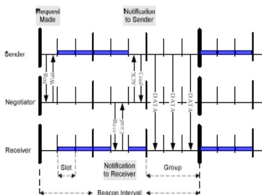
**Figure1: Time slot and channel negotiation in EMAC. Protocol signaling and data communication are indicated by vertical arrows. Horizontal blue line indicates when nodes are in sleep**
