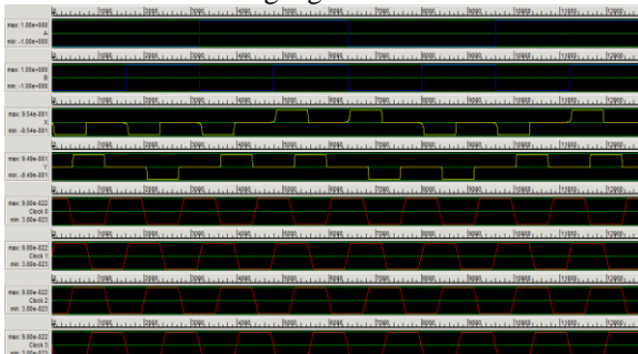
Fig1:Simulation of Feynman Gate in QCA
