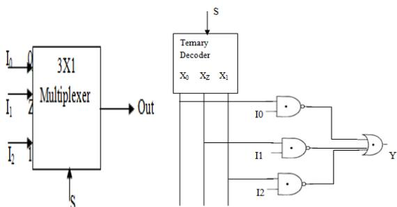
Figure 11: Block and circuit diagrams of 3X1 Ternary Multiplexer
