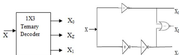
Figure 10: Block and Circuit diagram for 1X3 Ternary Decoder
