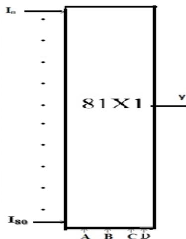
Figure 13: Block diagram of 81x1 Ternary Multiplexer
