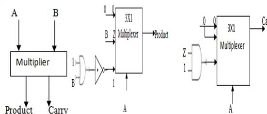
Figure 7: Block and circuit diagrams for one bit Ternary Multiplier
