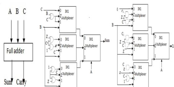
Figure 5: Block and circuit Diagrams for Ternary Full adder
