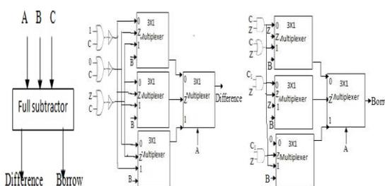
Figure 6: Block and circuit Diagrams for Ternary Full subtractor
