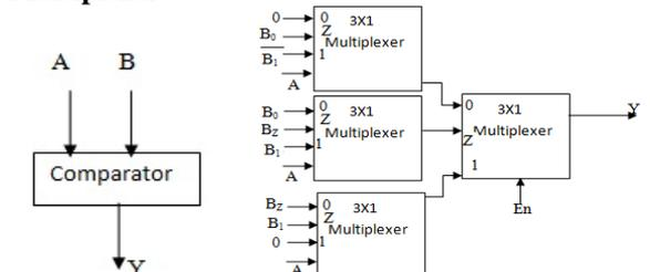
Figure 8: Block and circuit diagram for one bit Ternary comparator
