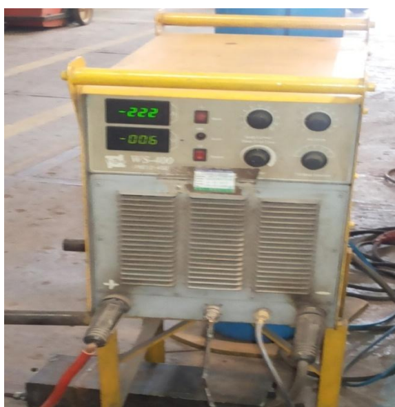
Figure 3: Shielded Metal Arc Welding Machine (Warp Engineering Model WS-400)
