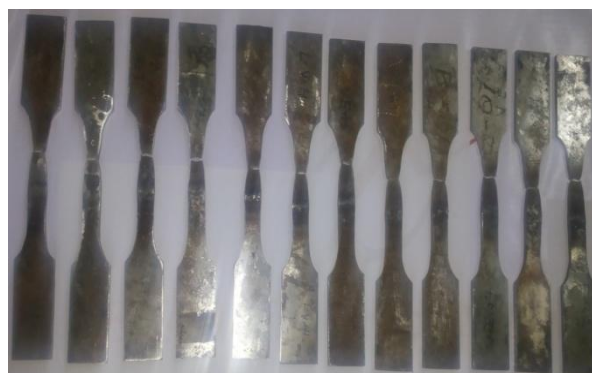
Figure 4: Broken Test Samples after Tensile Tests
