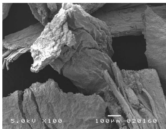
**Fig17. Typical SEM micrograph of the particles of waste tea after adsorption**
