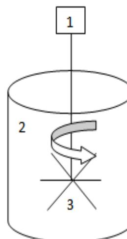
1. Electrical pump, 2. Container for batch study, 3. Agitator/ stirrer.
