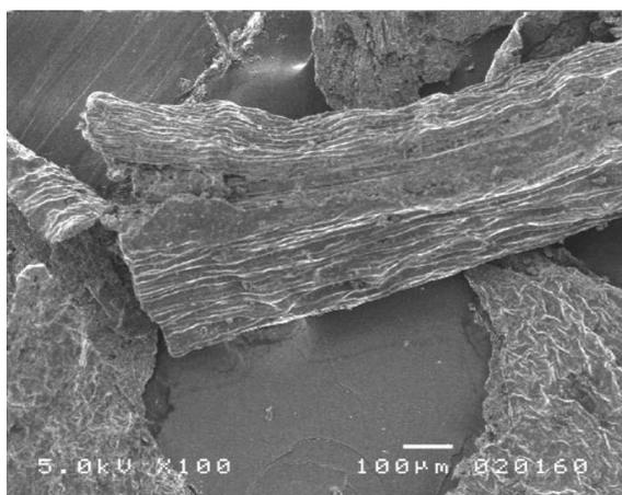
**Fig16. Typical SEM micrograph for the particles of waste tea before adsorption [21].**
