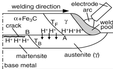
Fig. 10 Diffusion of hydrogen from weld metal to HAZ during welding [15].
