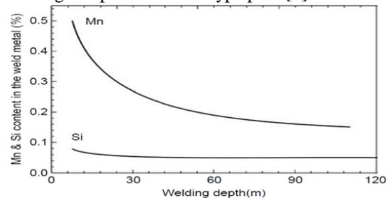
Fig. 9 Influence of depth of underwater welding on the content of elements in the weld deposit [1].
