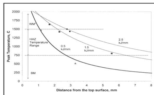
Fig. 4 Peak temperature profiles weighted and fitted for different weld samples; heat input values 0.5, 1.5, 2.5 kJ/mm [9].
