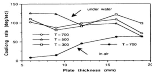
Fig. 3 Cooling rates for wet welding compared with welding in air [7].
