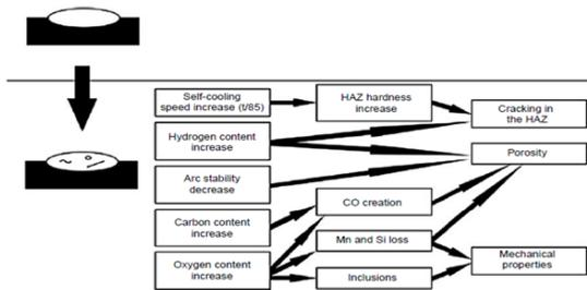
Fig. 1 The effect of moving the welding process to water environment [1].
