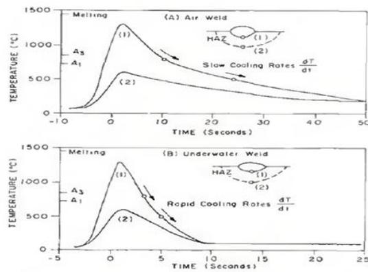
Fig. 6 Temperature histories of air welds compared to those of underwater welds [6].
