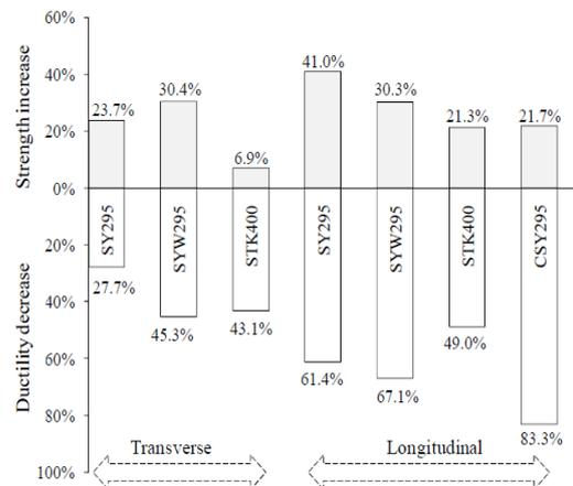
Fig. 11 Relative changes of strength and ductility from air welds to underwater welds [16]
