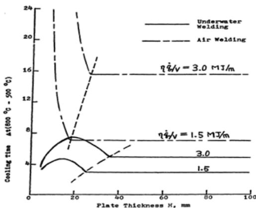
Fig. 5 Cooling time vs. plate thickness in wet and dry welds for two heat input values [4].
