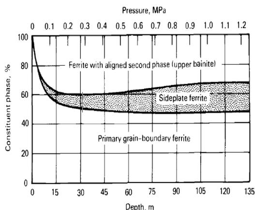
Fig. 8 Percentage of weld metal microstructural constituents for wet underwater welds as a function of water [8].
