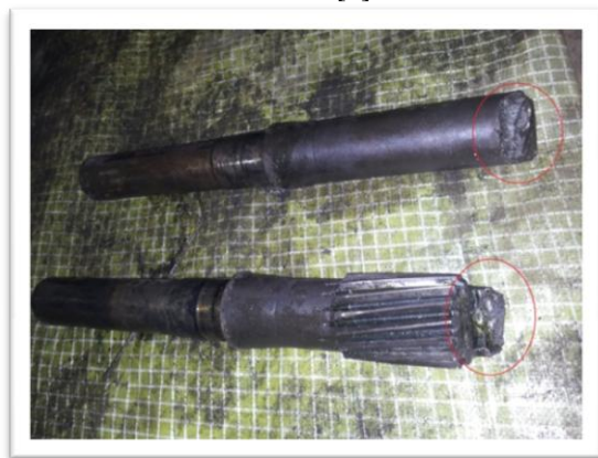
Figure 2: Failure of shaft
