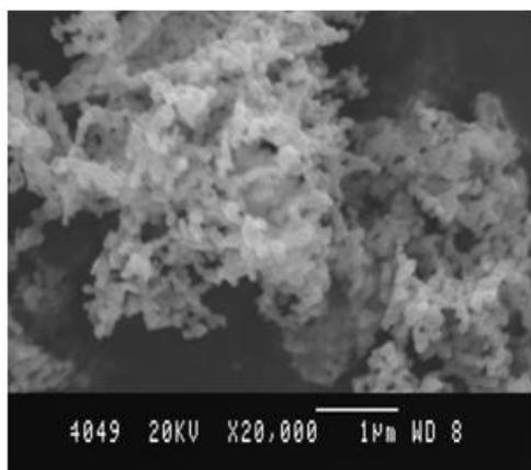
Figure 4: SEM of combustion synthesized ZnO nanoparticles
