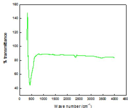
**Figure 3:** The FTIR spectra of combustion synthesized ZnO nanoparticles
