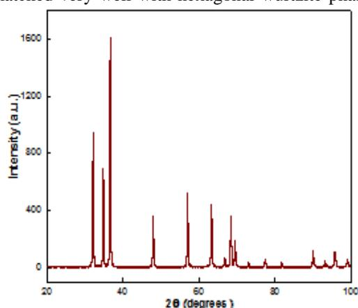
**Figure 1:** The powder X-ray diffraction pattern (XRD) patterns of the combustion synthesized ZnO nanoparticles
