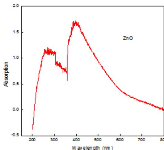
**Figure 2:** The UV-Vis spectrum of combustion synthesized ZnO nanoparticles
