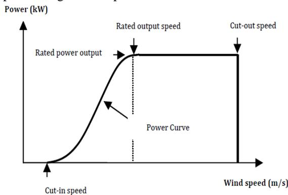
Fig: 3 Power from wind turbine
