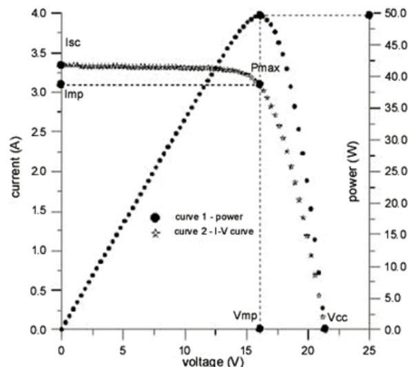
Fig: 2 VI and PV characteristics of solar cell
