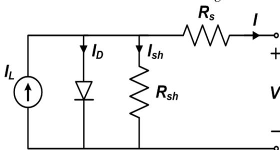
Fig: 1 Single diode model of solar cell
