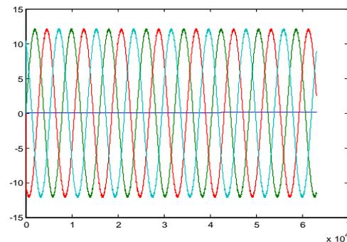
Fig: 7 Injected three phase generator current of wind generator (simultaneous operation with wind and PV)
