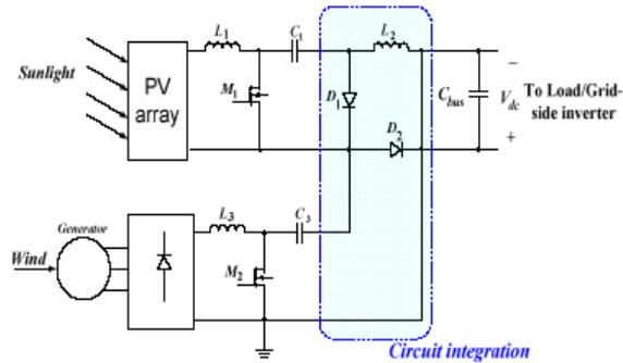
Fig: 6 proposed rectifier stage for hybrid wind/PV system
