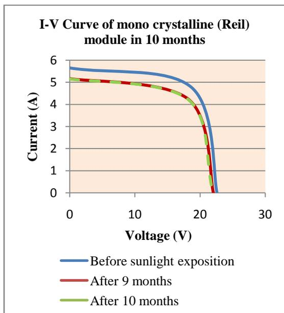
**Figure 7 Initial power stabilization in mono crystalline (Reil) module tested in NISE**
