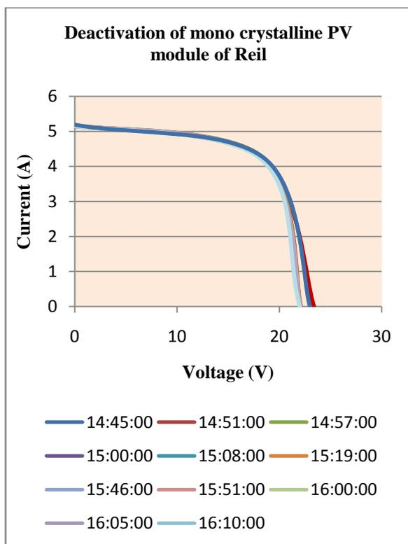
**Figure 24 Deactivation of mono crystalline PV module of Reil along 2 hours**
