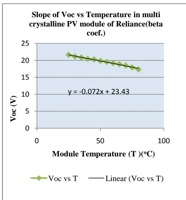
**Figure 11 Temperature coefficient for Voc of Multi C-Si PV module of Reliance (beta coef)**
