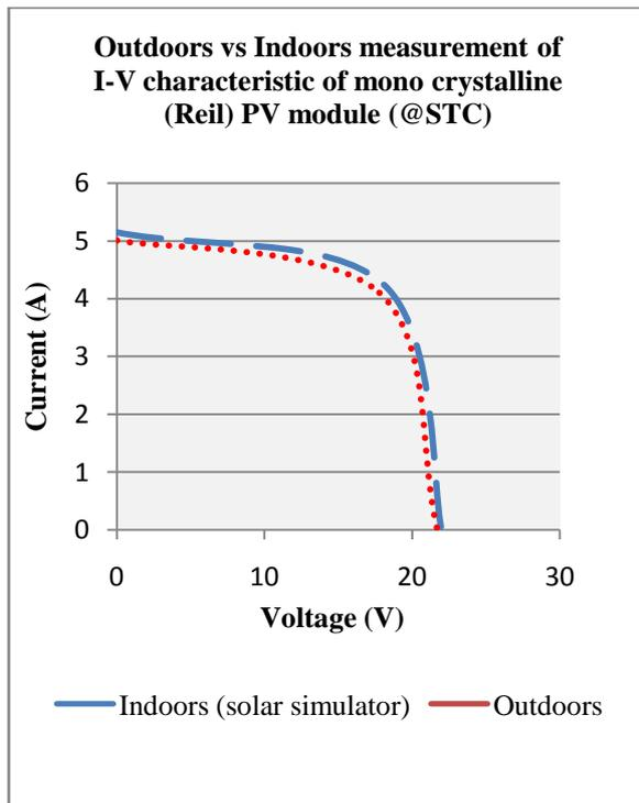
Figure 21 Comparison of outdoor and indoor measurement of I-V characteristic of a mono crystalline (Reil) PV module at STC after sunlight activation
