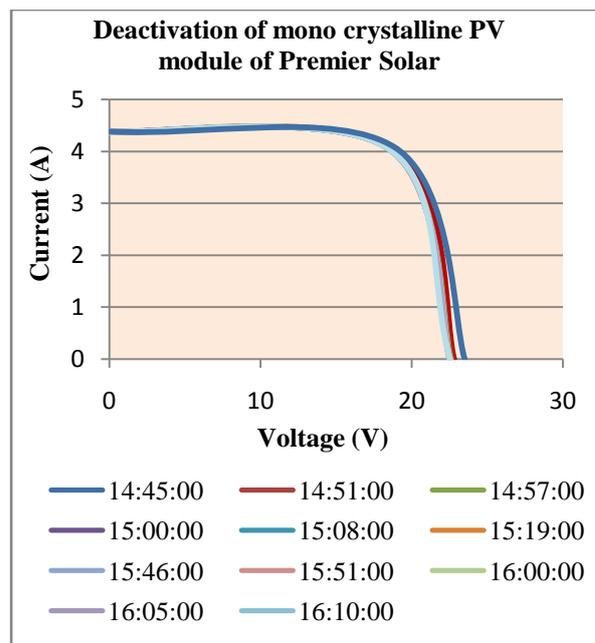
Figure 23 Deactivation of mono crystalline PV module of Premier Solar along 2 hours
