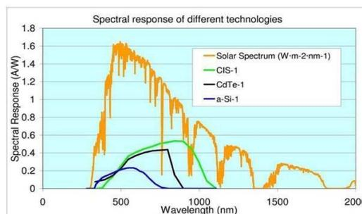
**Figure 2 Typical spectral responses of different thin film technologies and AM 1.5 spectral distribution**
