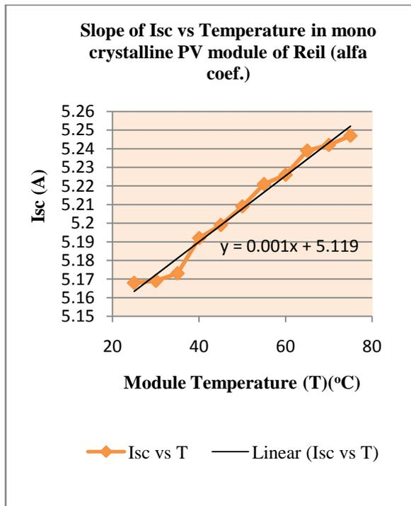
Figure 16 Temperature coefficient for Isc of Mono C-Si PV module of Reil (alfa coef)
