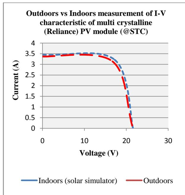
Figure 19 Comparison of outdoor and indoor measurement of I-V characteristic of multi crystalline (Reliance) PV module at STC after sunlight activation
