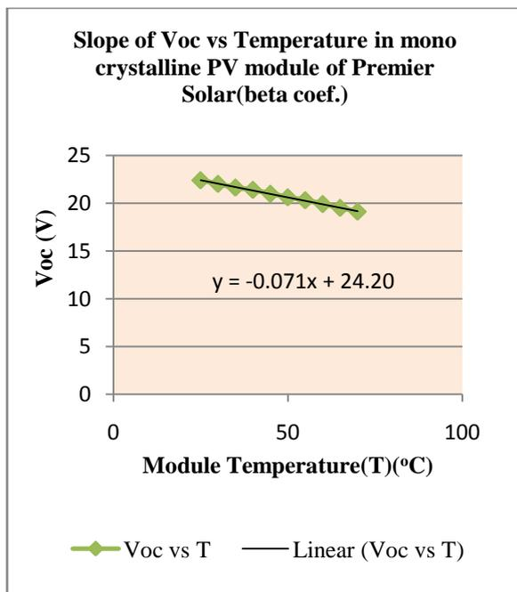
Figure 17 Temperature coefficient for Voc of Mono C-Si PV module of Premier Solar (beta coef)
