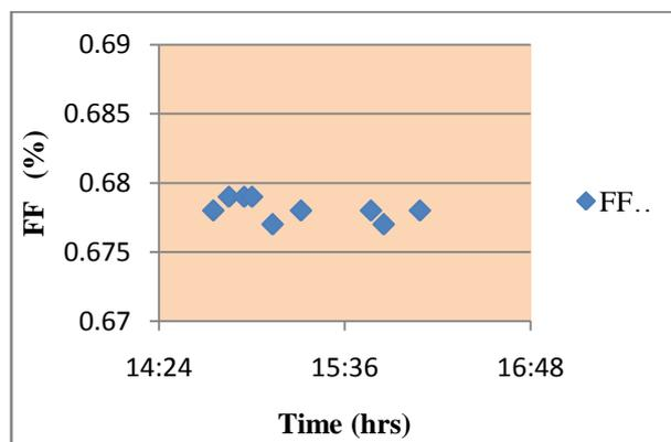
**Figure 27 Deactivation effect over FF (%) parameter in mono crystalline PV module of Reil along 2 hours**
