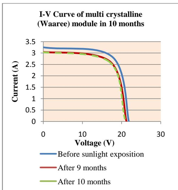
**Figure 10 Initial power stabilization of multi crystalline (Waaree) module tested in NISE**
