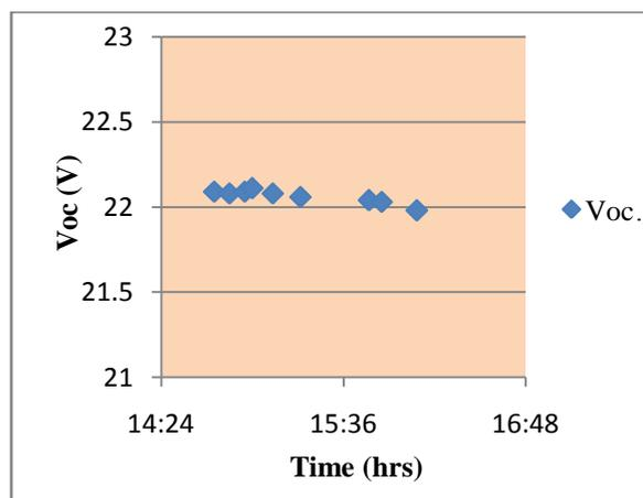
**Figure 26 Deactivation effect over Voc (V) parameter in mono crystalline PV module of Reil along 2 hours**
