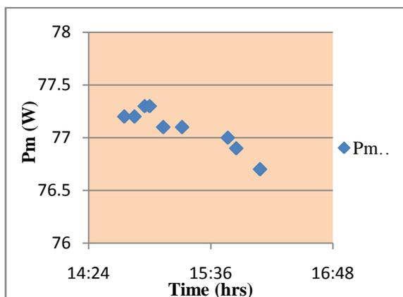
**Figure 25 Deactivation effect over Pm (W) parameter in mono crystalline PV module of Reil along 2 hours**
