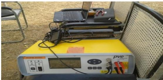
**Figure 6 Peak Power Measuring Device Tracer (PVPM 2540)**
