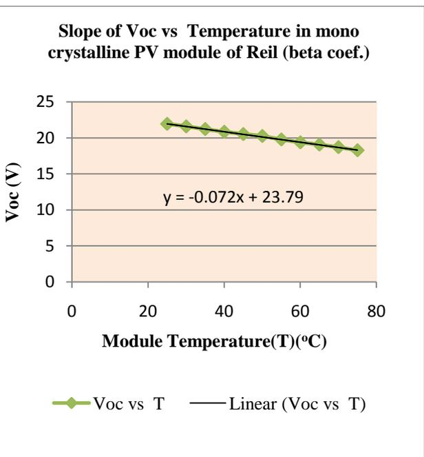
Figure 15 Temperature coefficient for Voc of Mono C-Si PV module of Reil (beta coef)
