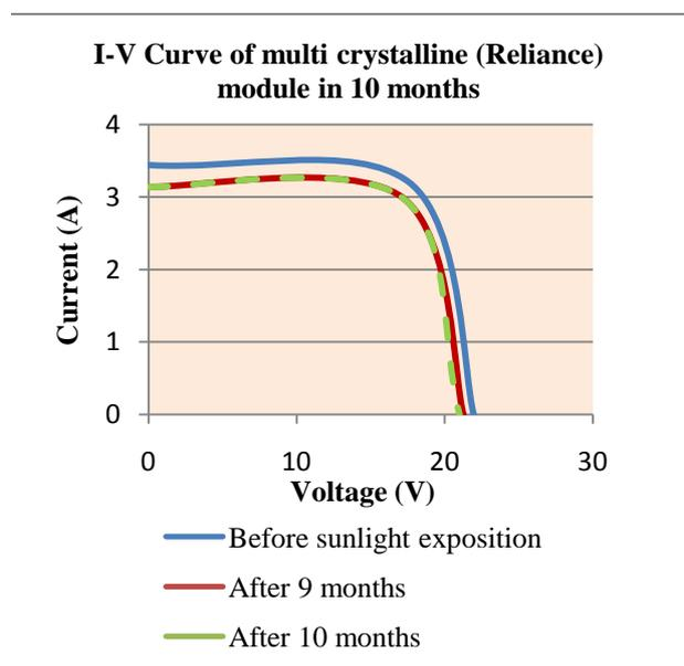
**Figure 9 Initial power stabilization multi crystalline (Reliance) module tested in NISE**
