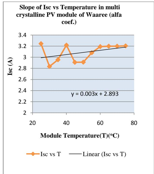
Figure 14 Temperature coefficient for Isc of Multi C-Si PV module of Waaree (alfa coef)
