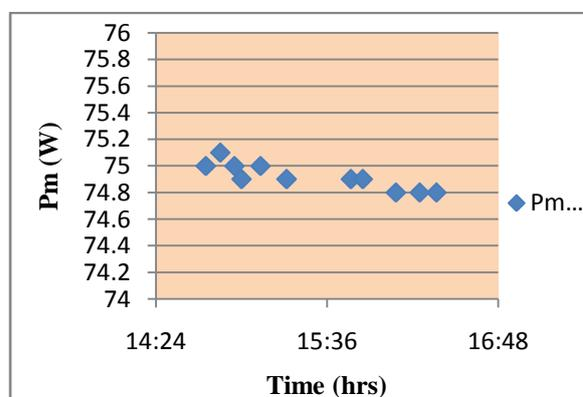
**Figure 28 Deactivation effect over Pm (W) parameter in mono crystalline PV module of Premier Solar along 2 hours**
