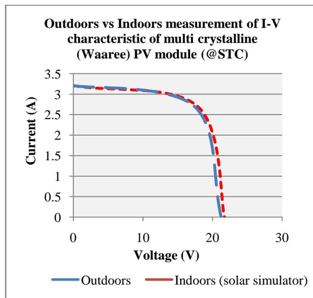
Figure 20 Comparison of outdoor and indoor measurement of I-V characteristic of multi crystalline (Waaree) PV module at STC after sunlight activation
