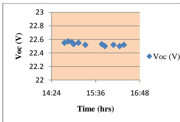
**Figure 29 Deactivation effect over Voc (V) parameter in mono crystalline PV module of Premier Solar along 2 hours**
