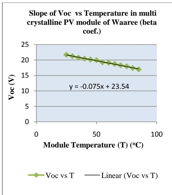
Figure 13 Temperature coefficient for Voc of Multi C-Si PV module of Waaree (beta coef)
