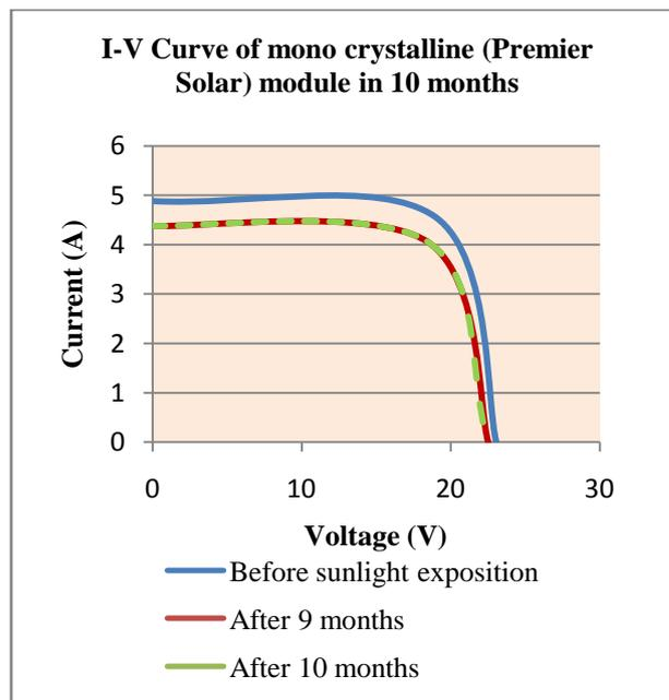
**Figure 8 Initial power stabilization in mono crystalline (Premier Solar) module tested in NISE**
