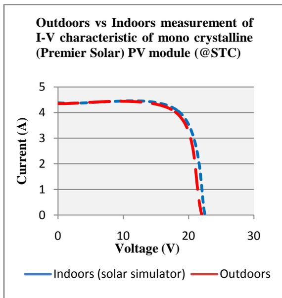
Figure 22 Comparison of outdoor and indoor measurement of I-V characteristic of a mono crystalline (Premier Solar) at STC after sunlight activation
