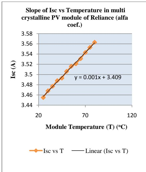
Figure 12 Temperature coefficient for Isc of Multi C-Si PV module of Reliance (alfa coef)
