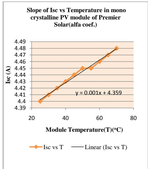
Figure 18 Temperature coefficient for Isc of Mono C-Si PV module of Premier Solar (alfa coef)
