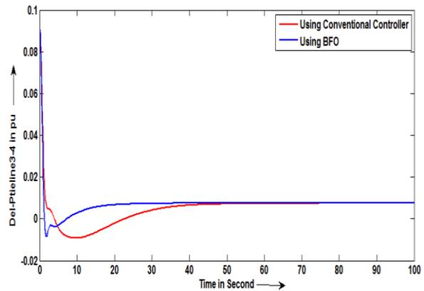
Figure 13 Del Tie line 3-4 with and without BFO
