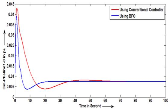
Figure9 Del Tie line 1-3 with and without BFO
