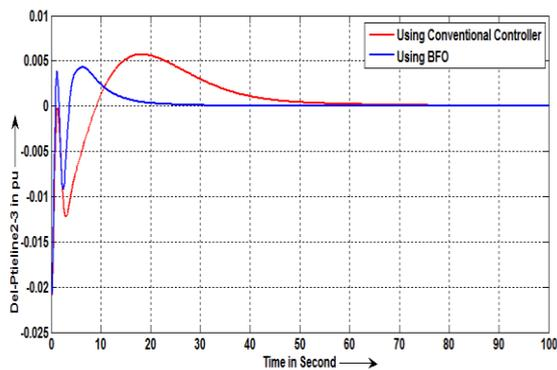
Figure 11 DelTie line2-3 with and without BFO
