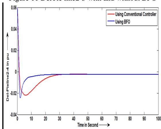
Figure 12Del Tie 2-4 with and without BFO
