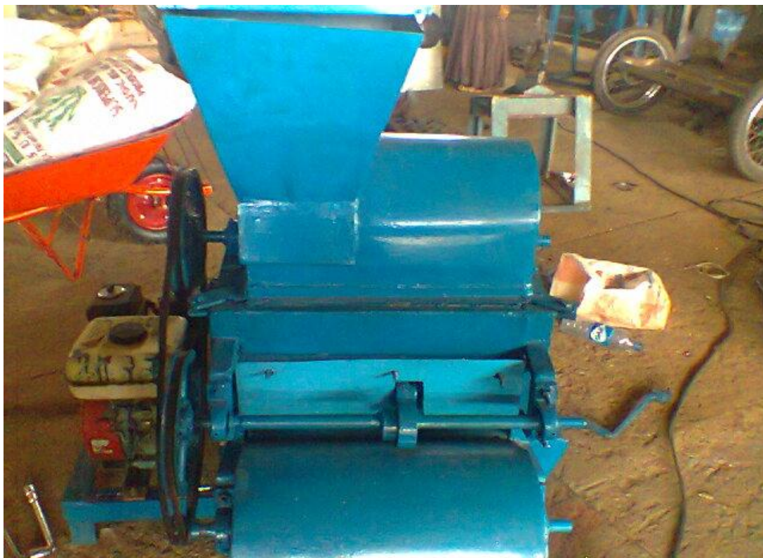
Plate 2: Front view of the Constructed Coffee Threshing Machine
