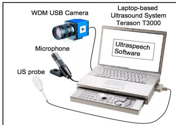
Figure 3 shows a typical ultrasound SSI system
