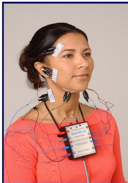
Fig 2: Electromyographic sensors attached to the face[11]
