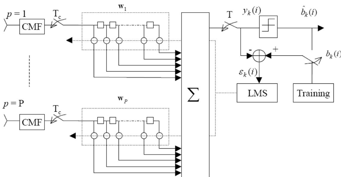
Figure 2: Structure of an adaptive MMSE space-time multiuser detector
