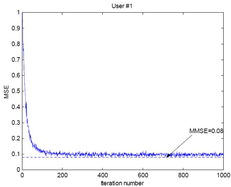
Figure 3. Convergence of the decentralized adaptive MMSE space-time multiuser detector
