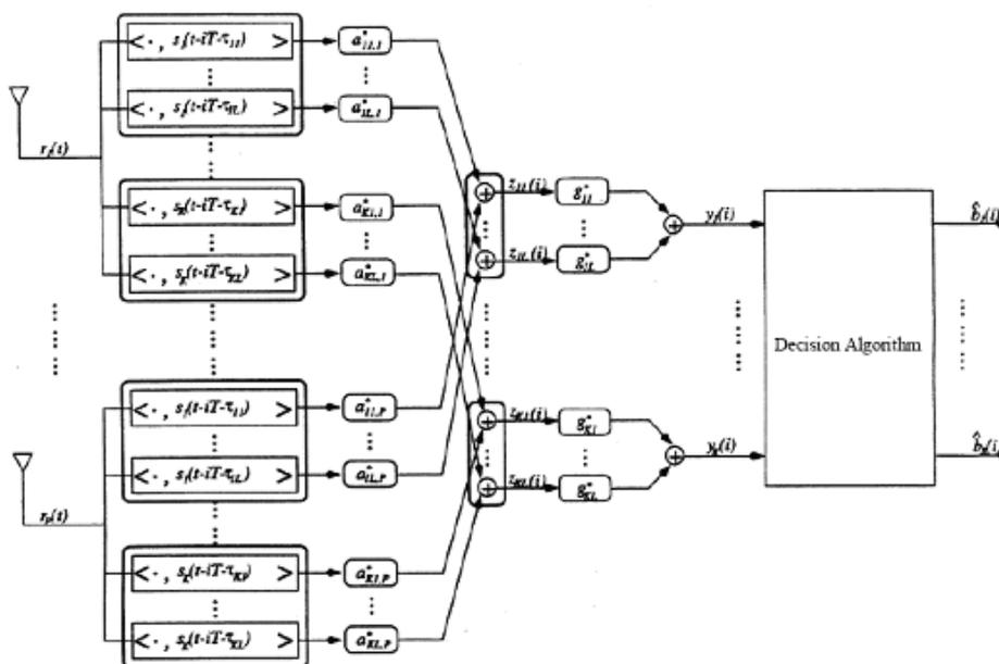
Figure 1: A conventional space-time multiuser receiver structure
