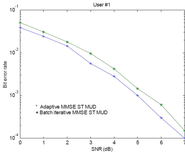
Figure 4. Bit error rate of the decentralized adaptive MMSE space-time multiuser detector in the steady state
