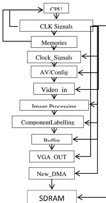
Figure 2. Top and linked levels diagram FPGA.
