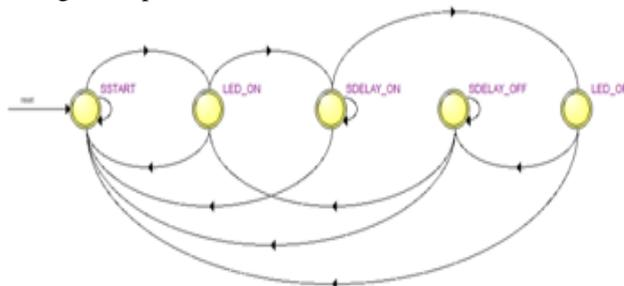
Figure 3. Ledblink finite state machine.
