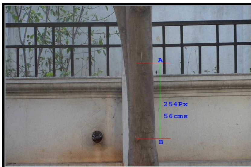
Fig-03: Mapping Digital pixel to the real world length.
