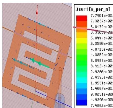
Figure 14: Current distribution at vector\_Jsurf
