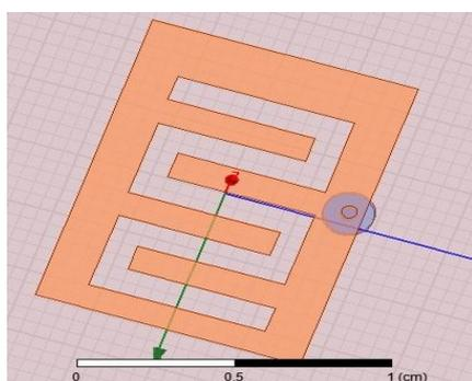
Figure 1: geometry of rectangular probe-fed with folded dipole.
