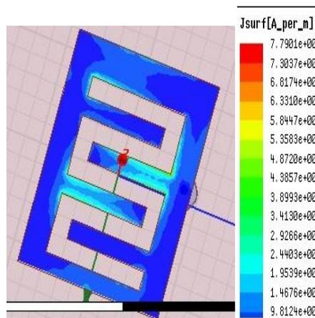
Figure 13: Current distribution at mag\_Jsurf
