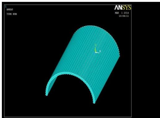
Fig. 1 Pipe roof model in ANSYS
