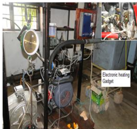
Fig.3 Experimental test rig set up with inset of online electrical heating
