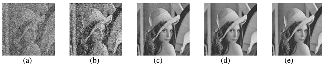
Figure 3.7: result for lena image of size 512x512 at 60% noise density (a) noisy image (b) MF output (c) DBA output (d) DBUTMF output (e) MDBMMF output (proposed algorithm).
