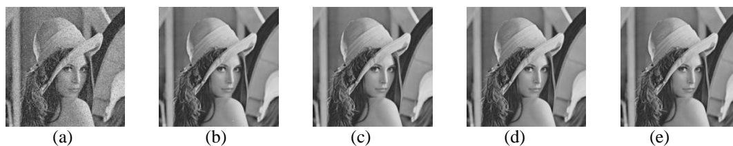
Figure 3.5: result for lena image of size 512x512 at 10% noise density (a) noisy image (b) MF output (c) DBA output (d) DBUTMF output (e) MDBMMF output (proposed algorithm).
