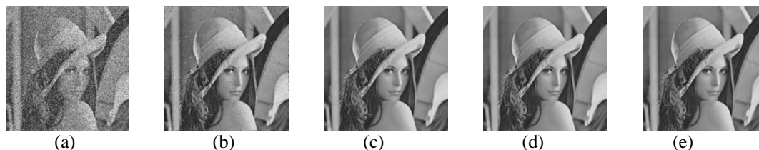
Figure 3.6: result for lena image of size 512x512 at 30% noise density (a) noisy image (b) MF output (c) DBA output (d) DBUTMF output (e) MDBMMF output (proposed algorithm).
