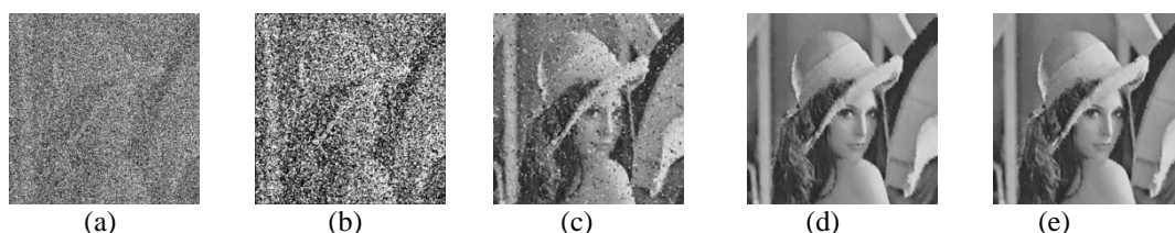
Figure 3.8: result for lena image of size 512x512 at 80% noise density (a) noisy image (b) MF output (c) DBA output (d) DBUTMF output (e) MDBMMF output (proposed algorithm).
