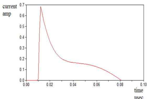
Fig.4. Magnified current response of the detailed transformer model
