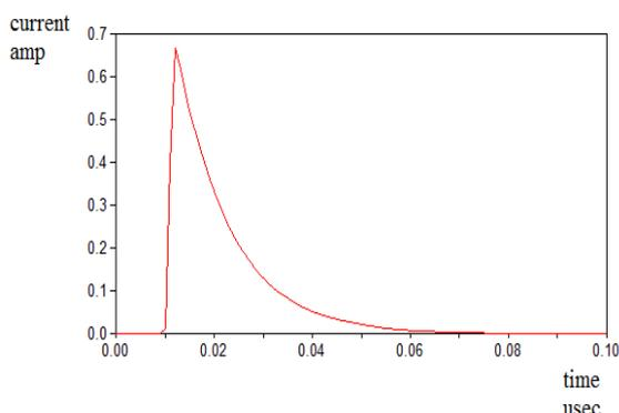
Fig.5. Current response of the reduced transformer model
