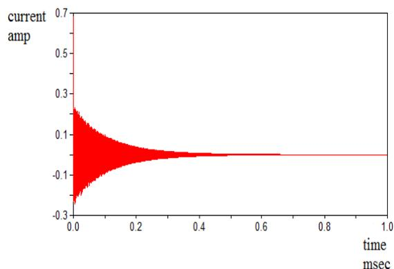
Fig.3. Current response of the detailed transformer model
