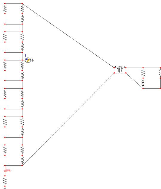
Fig.2. Reduced transformer modeled in ATP Draw
