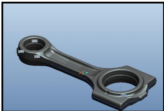
Fig -2: Model of Connecting rod
