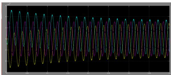
Voltage  $V_{abc}$  after harmonic correction(Y axis – Voltage in V, X axis - time in millisecond)
