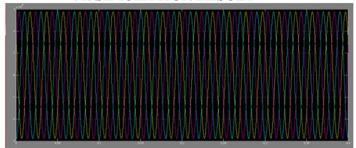
Voltage *Vabc* without Harmonic Correction(Y axis – Voltage in V, X axis - time in millisecond)
