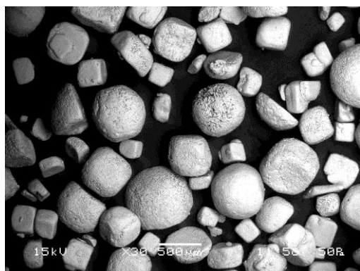
Sodium chloride before spray drying Sodium chloride after spray drying (Spray dried mixture of NaCl collected in the cyclone separator operated at T_i = 120\text{ }^\circ\text{C} , U_{asp} = 0.00478\text{ kg/cm}^2 , U_p = 2.279604\text{ ml/min} , C_s = 1\text{ gm/ml} , P_{i\text{-air}} = 2.10919\text{ kg/cm}^2 )
