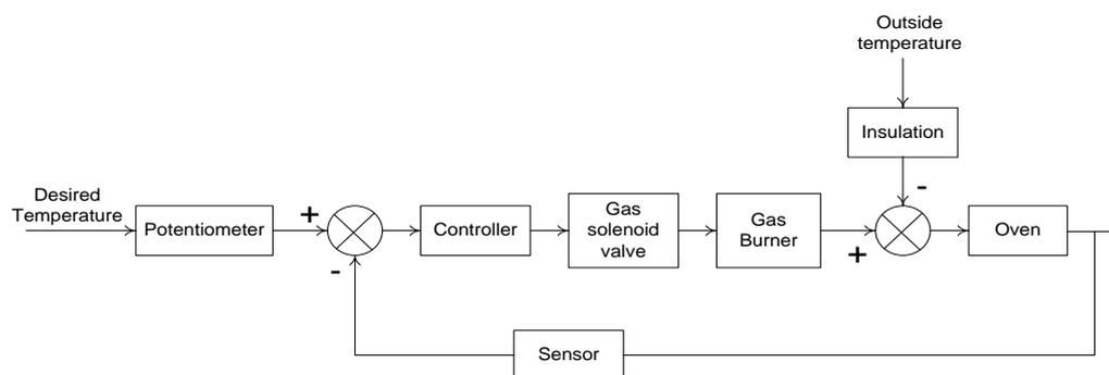
Figure 2: Block Diagram of OTC System
