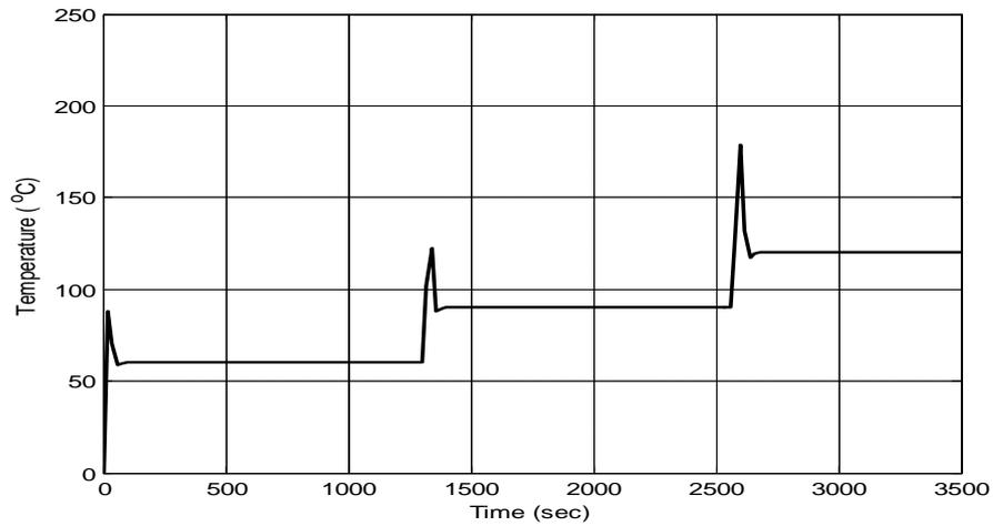
Figure 7: Simulation Result of PID control for Skogestad Method
