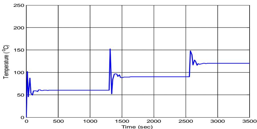
**Figure 5: Simulation Result of PID control for Ziegler-Nichols' Closed Loop Method**
