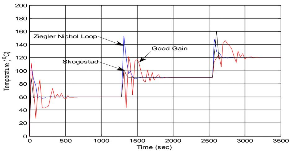
Figure 8: Comparison of the simulation Results over entire experimental period
