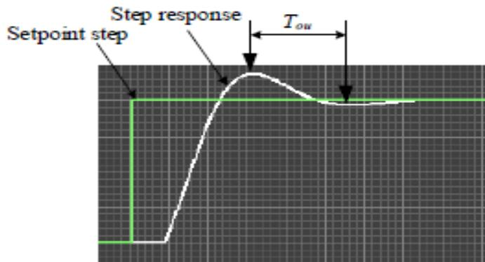
**Figure 3: Reading off the time between the first overshoot and the first undershoot of the step response with P controller**
